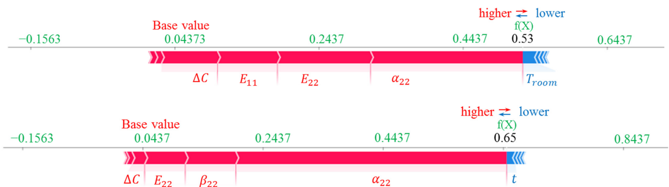
Figure 10. SHAP force plots for two different samples for the prediction of \kappa_{yy}^0 .
